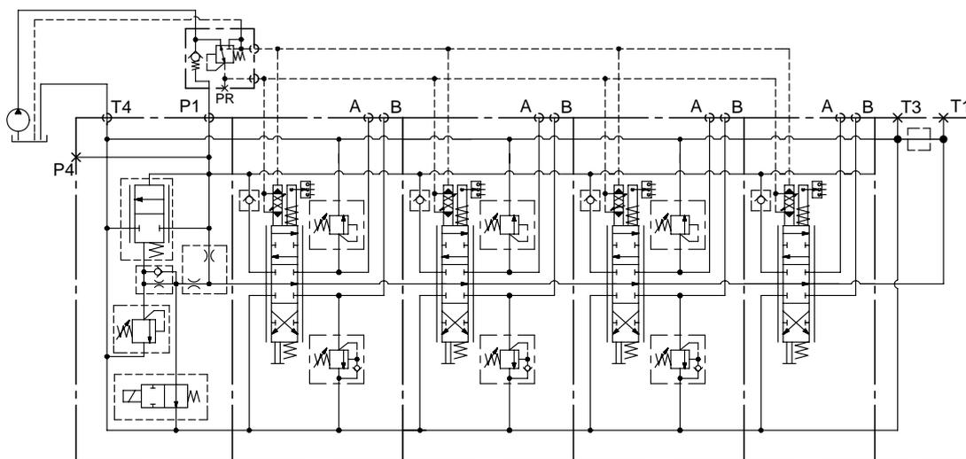
The circuit diagram shows a complete RS 210 valve, 4 sections with an inlet with flow regulator ("Q-inlet") and completed with pilot supply and spool controls for remote control.
