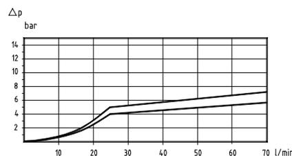
Pressure drop, P1 -T4, inlet I02Q/I06Q, with flow control FKA283/2 and PF12, outlet U01B
