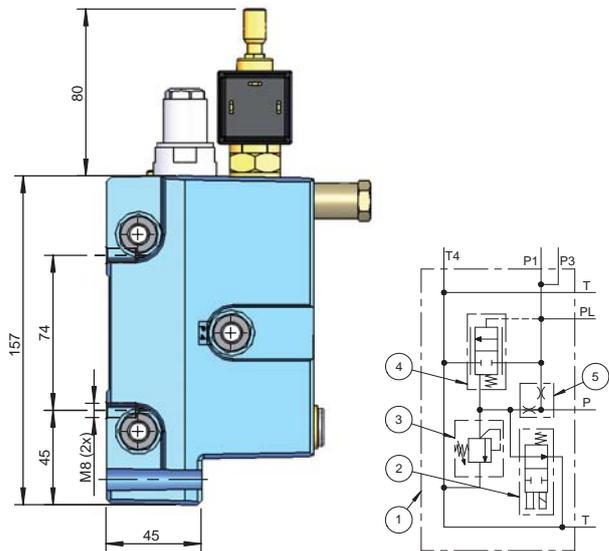
**I02Q** is an inlet section with flow control, main relief valve and unloading function.
