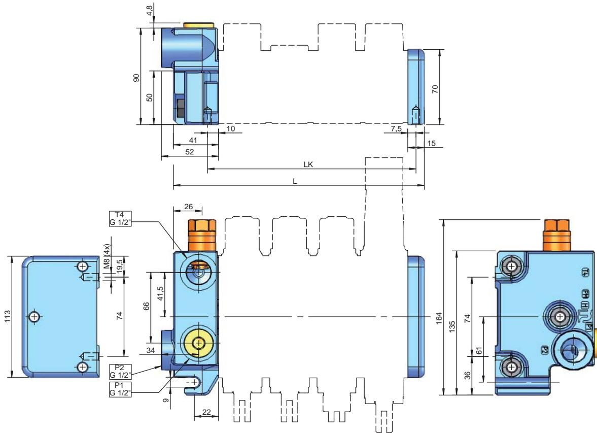
**I02C** has two pump ports and one tank port. The main relief valve cavity is on the A-side.
